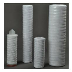
SS Filters Wound Filter Cartridges are manufactured using a high speed, continuous wind process which creates a superior one-piece filter with hundreds of diamond shaped tunnels that get progressively smaller from the outer diameter to the core. Finer particles are progressively trapped as fluid travels to the centre of the filter allowing for much greater retention capacity than straight surface filter media of same dimensions & porosity.
