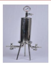
SS Filters stainless steel cartridge filter housings are designed for high purity applications. All wetted surfaces are constructed of SS 316 / SS 304 and are mirror polished, providing excellent corrosion resistance. The housing comes in 10" to 40"cartridge sizes to meet the needs of your application. The housing can support both Double Open End (DOE) and Code-7 type cartridges. The design of the housing provides for positive seal with the filters thereby preventing fluid by pass.
