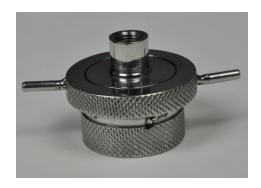
Stainless steel 47 mm Filter holder is designed for ultra-cleaning or sterilizing of gases or liquids under high or low pressure. The liquid is filtered through a 47mm disc filter of appropriate pore size by passing it through pressure pump. Gas can be directly passed through inlet.
